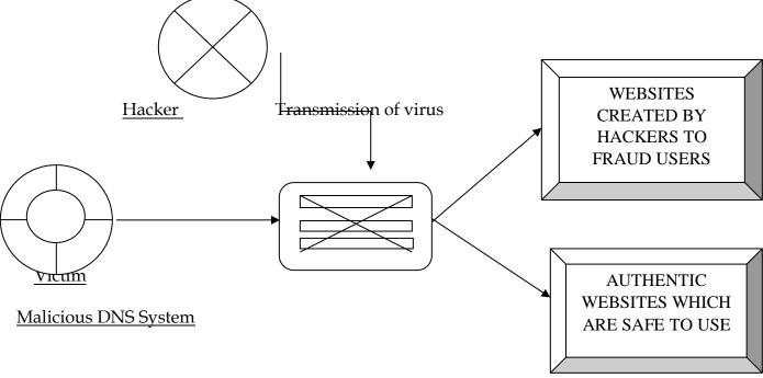
The above diagram depicts DNS (Domain Name System) hijacking where the malware replaces the router's DNS with malicious settings. Once the user's server is hijacked, even if the correct URL address is entered the user will be redirected to fake websites which will cause unusual tasks.
